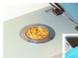
Portable a_w -measurement instrument LabSwift-aw
